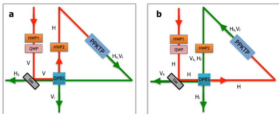
HWP: halfwave plate; QWP: quarterwave plate; DM: dichroic mirror; DPBS: dual polarizing beam splitter; PPKTP: non-linear crystal.
